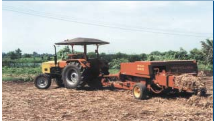
A field trial where New Holland balers, pulled by a tractor, haul cane residue and drop bales
