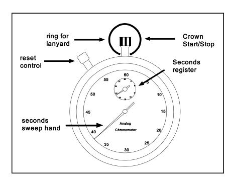
Figure 2. Type II stopwatch.
