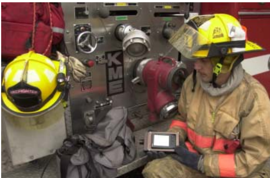
A handheld nuclear isotope detector, shown here with a Palm personal digital assistant interface, is designed for simple, widespread, first-responder use.
