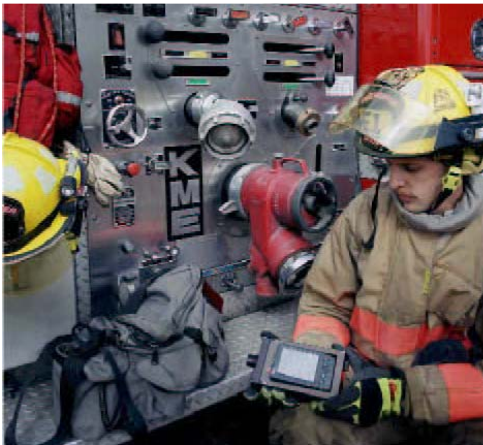
A Los Alamos firefighter holds the latest in nuclear detection and identification tools, a handheld spectrometer with a Personal Digital Assistant (PDA) as the interface for quick uploading of technical data right from the field.
