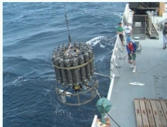
Launch of a conductivity-temperature-depth (CTD) sounder.
