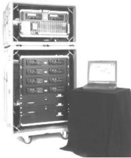
Figure 2-7. TRP-1000 transportable radio interconnect system, JPS
