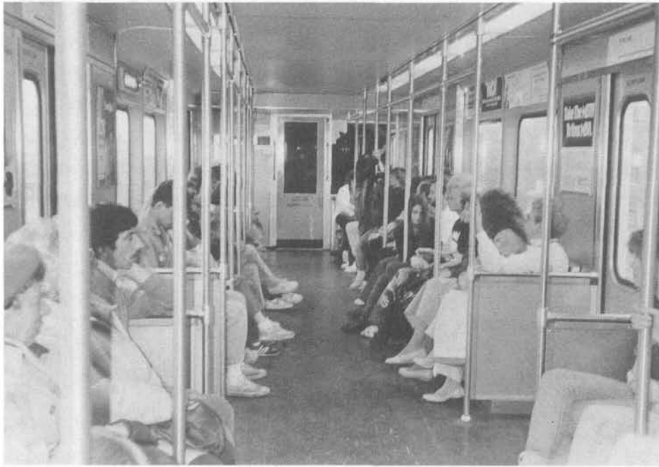
FIGURE 4-3. LONGITUDINAL ARRANGEMENT OF SEATS
