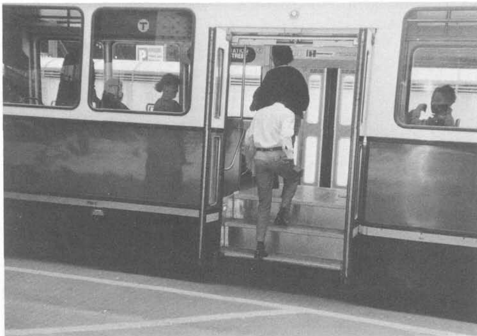
FIGURE 4-2. LOW-PLATFORM RAIL TRANSIT VEHICLE
