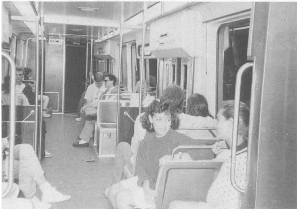
FIGURE 4-4. TRANSVERSE ARRANGEMENT OF SEATS
