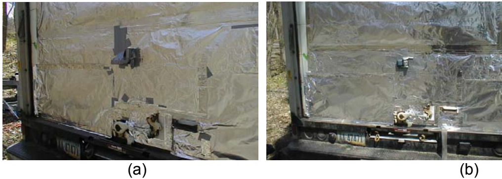
Figure D.1 Savi (a) and Hi-G-Tek (b) Seals Attached to Coated Roll-Up Door
