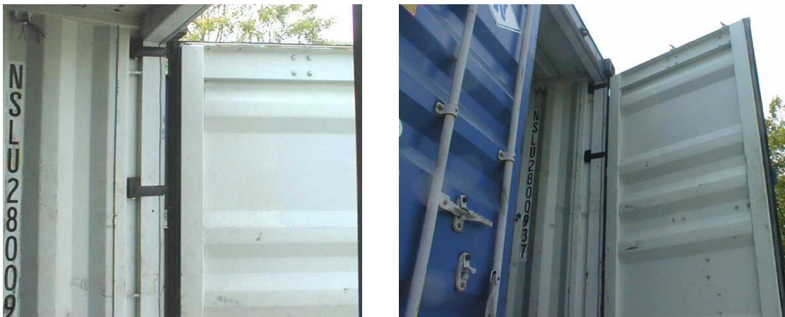
Figure B.30.c. Seals Mounted on Container Frame
