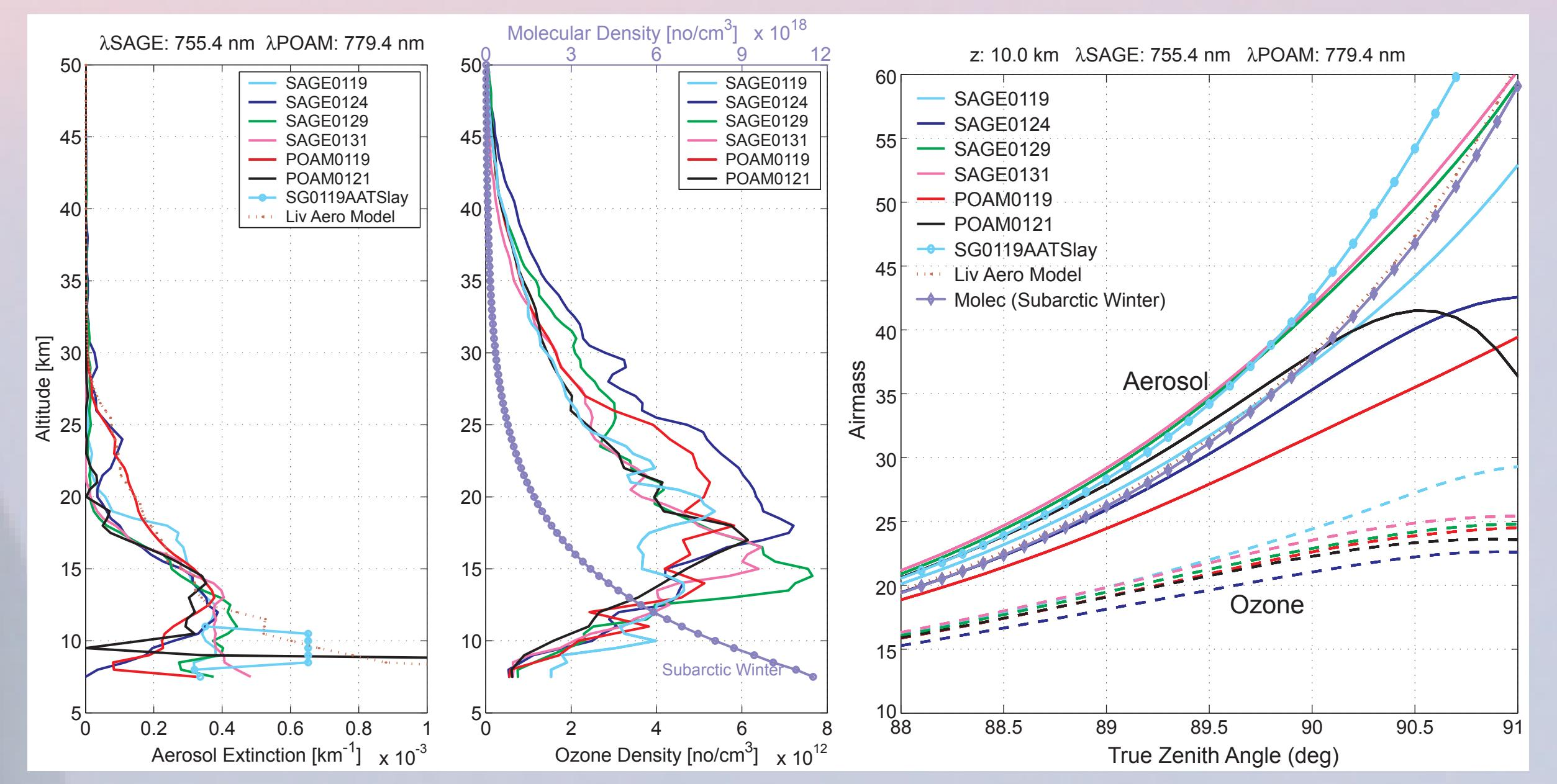
Airmass =  $\text{OD}_{\text{sun-viewing path}} / \text{OD}_{\text{vertical}}$ , assuming homogeneity in spherical shells
