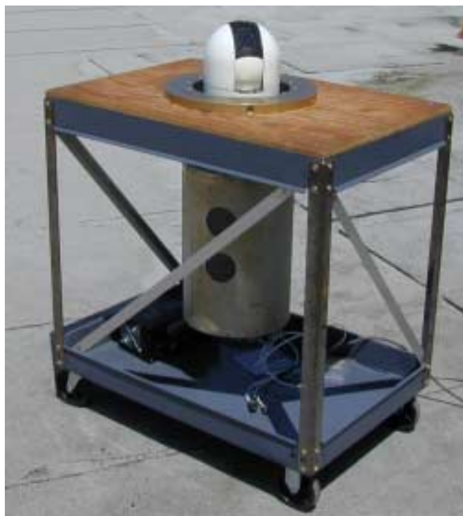
Figure 3. Fourteen-channel Ames Airborne Tracking Sunphotometer (AATS-14). Dimensions are in inches.
