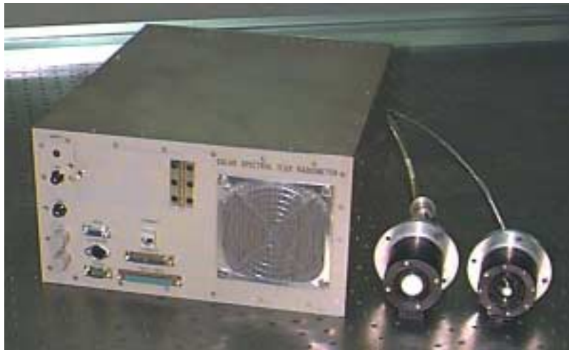
Figure 1: The Solar Spectral Flux Radiometer with detector heads for up – and downwelling radiation
