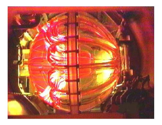
Liquid at rest in a transparent spherical tank under low gravity shows one aspect of the surprising behavior of fluid systems in space.
