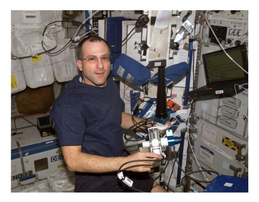
In this ISS onboard photo, Expedition Six Science Officer Donald R. Petit works to set up the Pulmonary Function in Flight (PuFF) experiment hardware in the Destiny Laboratory. The PuFF experiment was developed to better understand what effects long-term exposure to microgravity may have on the lungs.
