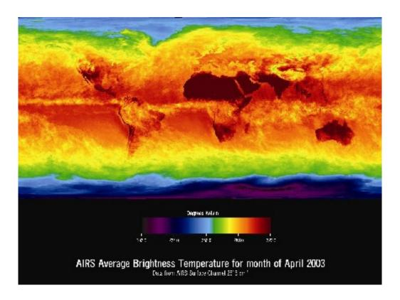
The Atmospheric Infrared Sounder (AIRS) and Advanced Microwave Sounding Unit (AMSU) instruments on the Aqua satellite are generating the most accurate, high resolution measurements ever taken from space of the infrared brightness (radiance) of Earth's atmosphere, yielding a global, three-dimensional map of atmospheric temperature and humidity.
