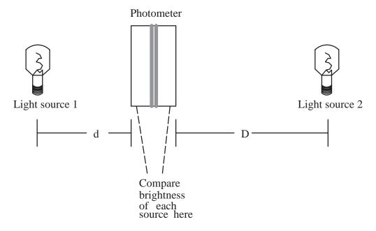
6. 2 equal wattage bulbs placed at the same distance should produce the same brightness in the photometer.
