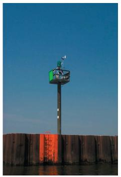
Meteorological station at Saugatuck Harbor Pier Light. Station is equipped with anemometer, wind direction vane, and phone model for data download.
