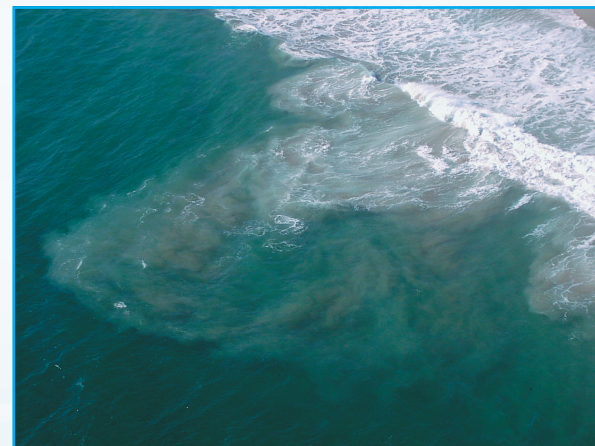
Rip currents often generate a plume of sediment moving away from shore.
