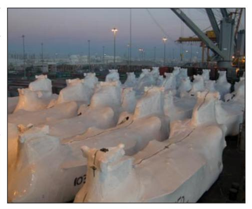
CH-47 Chinook helicopters from the 101st Airborne Division (Air Assault) are stored on the upper deck of the U.S.N.S. Benevidez for shipping back to the United States. The "shrink wrap" plastic coating is used to protect the aircraft from exposure to the salt air.
