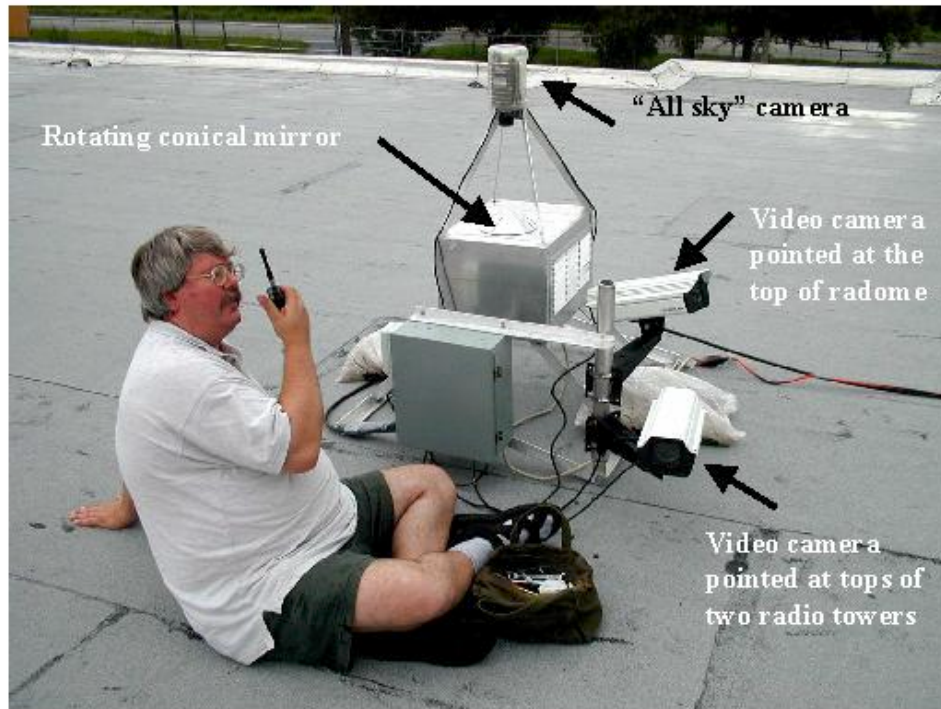
Figure 12. Setting up the video surveillance system at the WSR-88D site in Ruskin, FL, Summer 2000.
