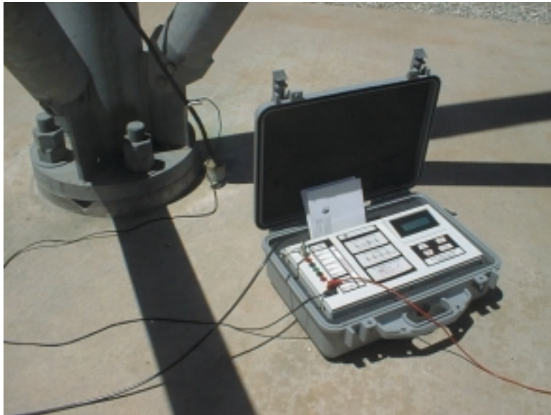
Figure 8. The ESA-1000, ready for measurements of the impulse impedance of a grounding point at a leg of the antenna tower.
