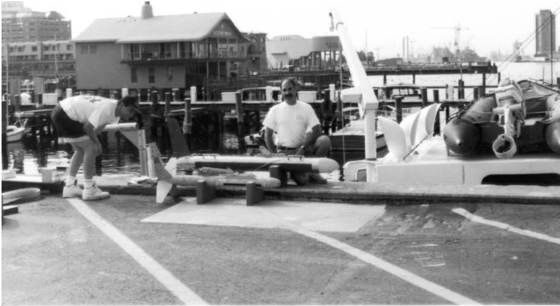
FIG. 7 High Speed, High Resolution Side Scan Sonar Towfish. A standard side scan sonar towfish is shown in the foreground for comparison.
