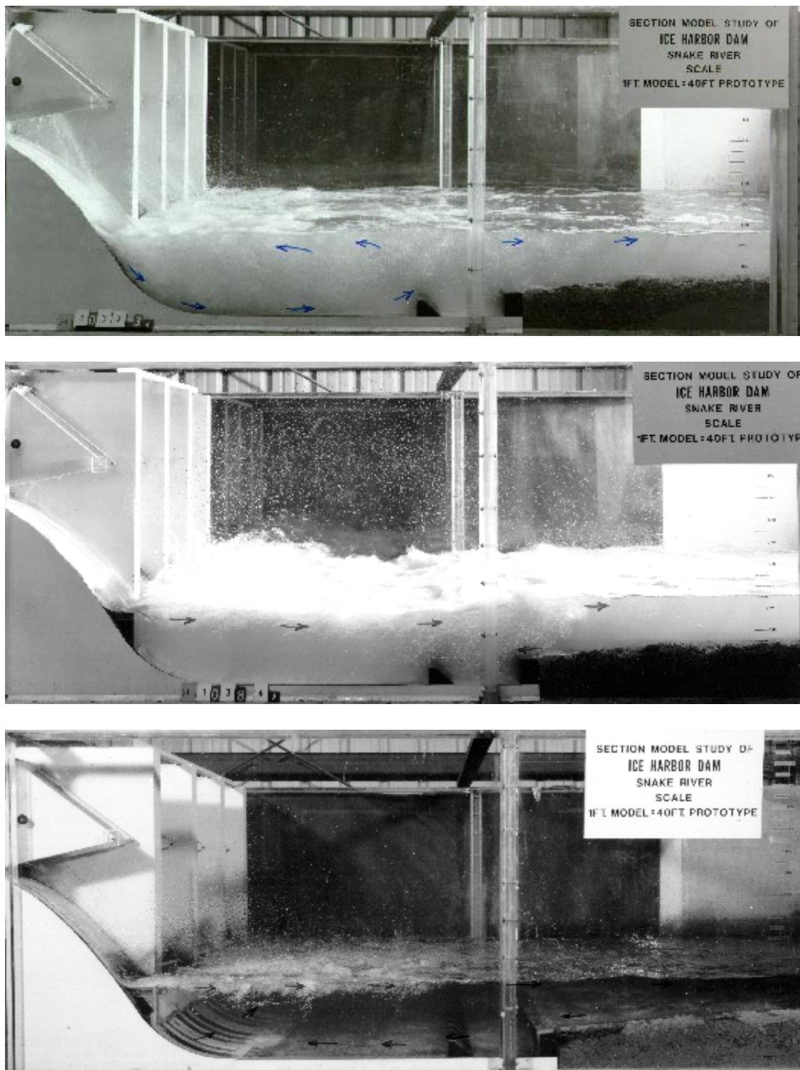
Figure 4-2. Ice Harbor Sectional Spillway Model - Visual Comparison of Non-deflected Spill, Deflected Spill, and Submerged Discharge
