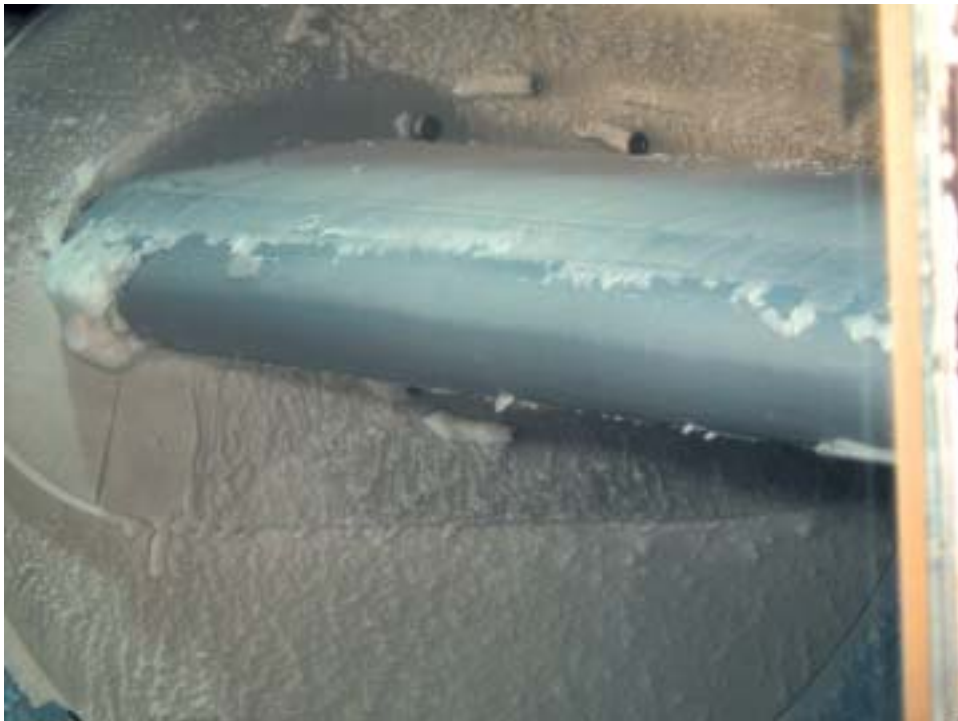
"The NASA-developed Electro Expulsive Separation System (EESS) is shown in a testing chamber where it proved it could rid aircraft from ice layers ranging from thin frosts to thick glazes."
