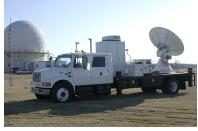
NSSL collaborated to build the SMART-Radar, a 5-cm mobile Doppler radar capable of scanning and penetrating an entire tornadic storm or hurricane.
