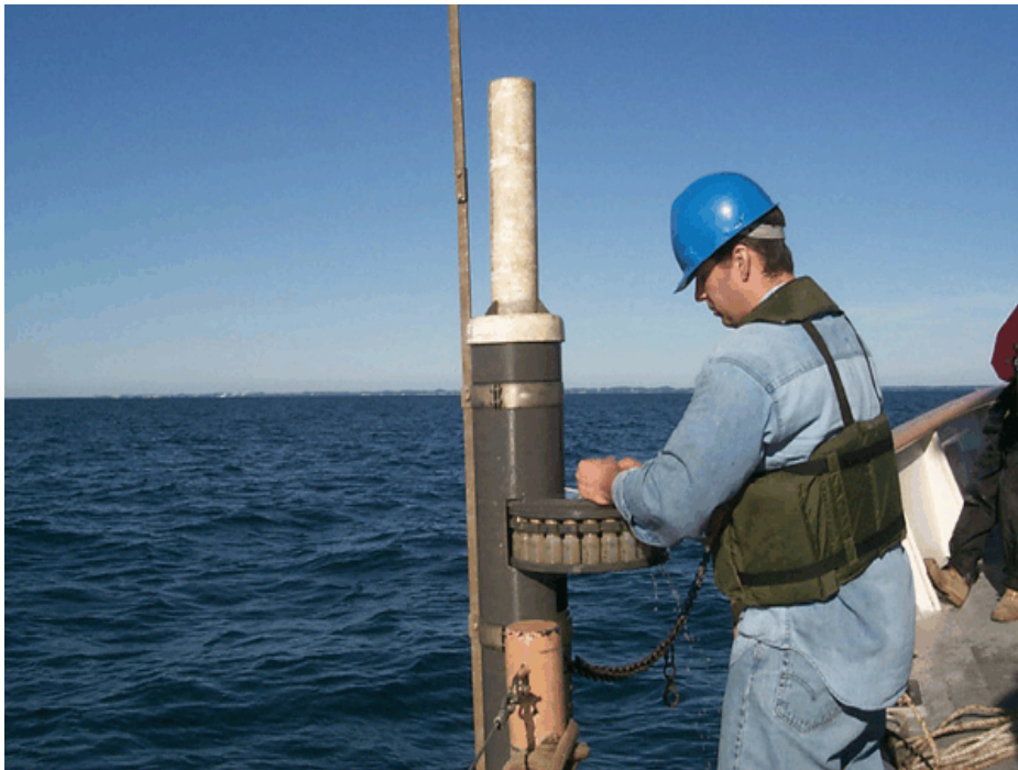
Retrieval of sequential sediment trap in southern Lake Michigan.
