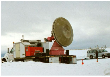
The OU Doppler-on-Wheels and the NSSL Mobile Laboratory take measurements of electrified snowstorms in Idaho during the Intermountain Precipitation Experiment.
