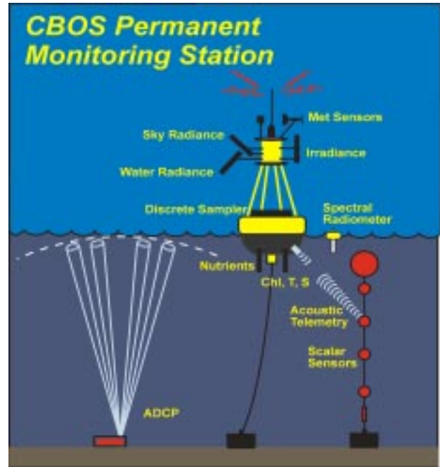
Schematic of monitoring equipment
