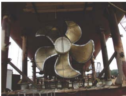
The ship's 14-foot propeller is designed for ultra-quiet operation and minimum cavitation
