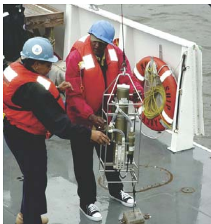
Deck crew prepares to lower the CTD to measure water conductivity and temperature at different depths
