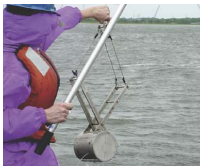
Using a bottom-grab instrument, a sediment sample is retrieved
