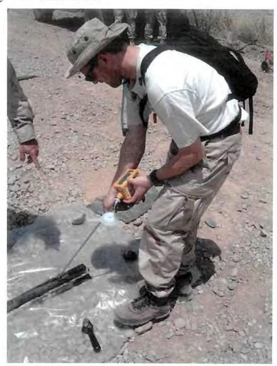
Figure D-14 (U): Screening Soil Sample With PID
