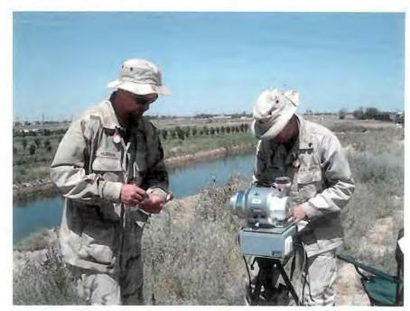
Figure D-5 (U): Air sampling for radioactive material
