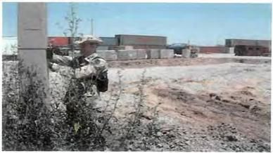
Figure D-20 (U): VOC Sampling in SSA Area / Exposed Soil Contamination Area
