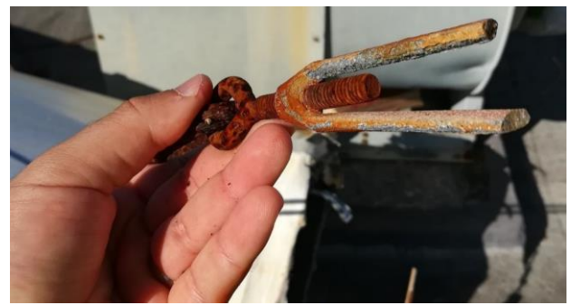
Figure 20. This corroded turnbuckle failed, allowing the boiler stacks shown in Figure 11 to topple.
