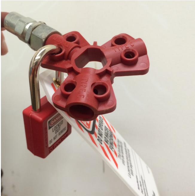
Two examples of the various lock-out, tag-out devices used on House equipment.
