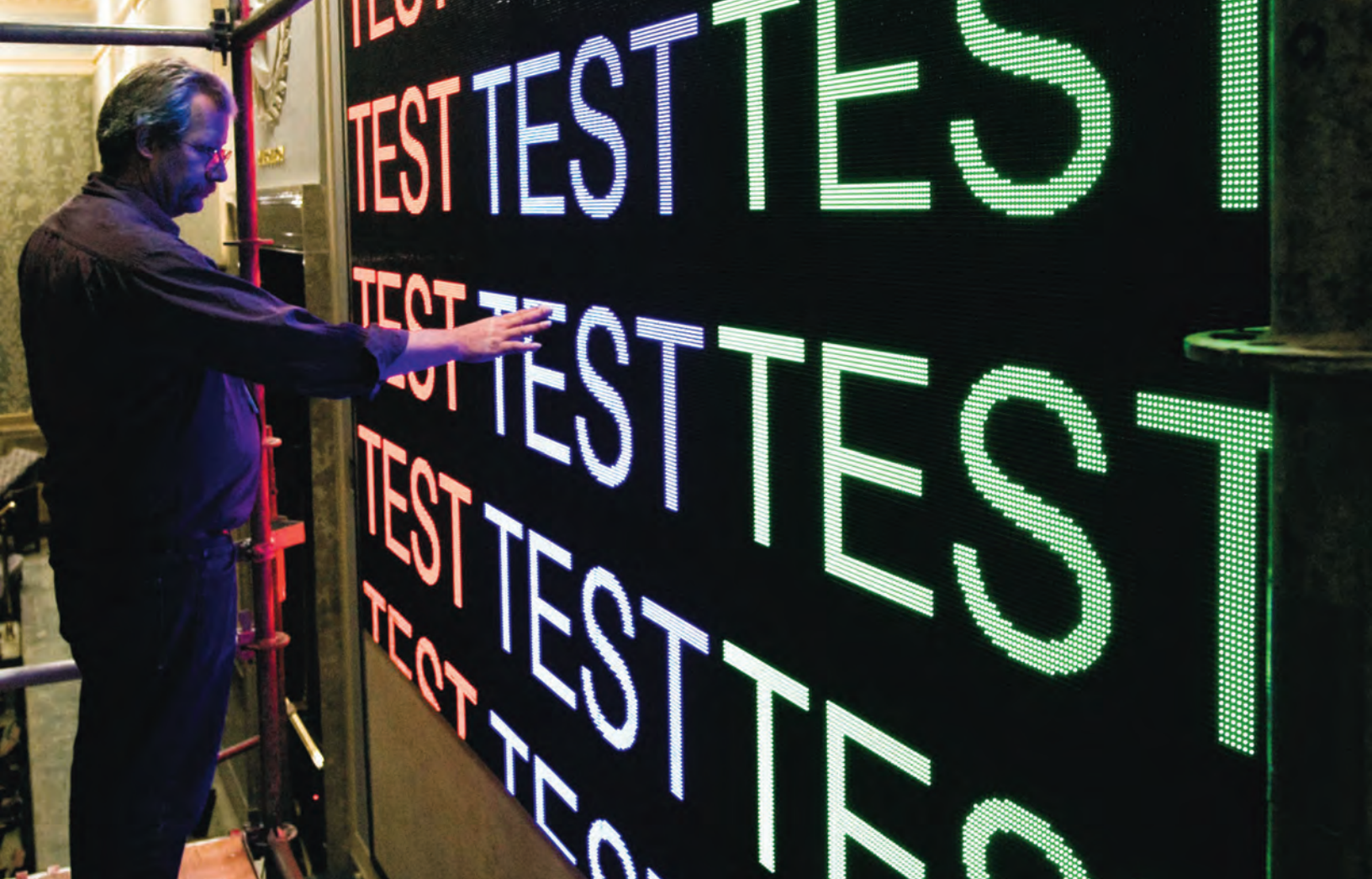
Testing the House Chamber Voting Display Board after installation in 2011. The House electronic voting system made votes more efficient, reducing the time one vote takes from 45 minutes to 15 minutes. Photo by Dewitt Roseborough
