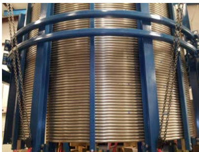
An 800-meter sample toroidal field conductor was delivered to the EU in June 2014. Photo: U.S. ITER
