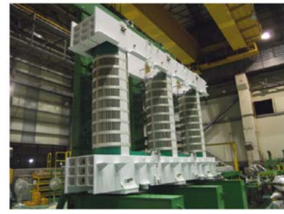
Laminated core of a high voltage substation transformer in fabrication for the steady state electrical network. Photo: Hyundai Heavy Industries
