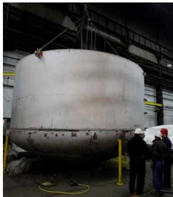
Joseph Oat Corporation in Camden, NJ is completing fabrication of drain tanks. Photo: U.S. ITER
