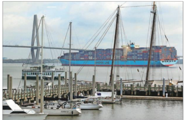
FILE/BRAD NETTLES/STAFF The shipping industry is shifting to larger, heavier vessels like the 1,155-foot-long Axel Maersk. The trend has some U.S. ports scrambling to deepen their navigation channels.
