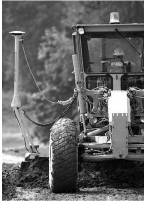
Motor grader with machine control.
