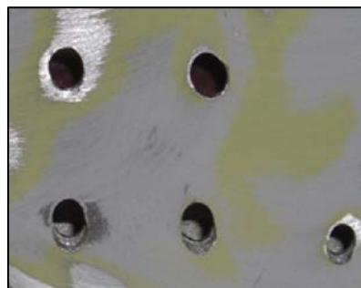
Figure 3 Oblong Holes of the DEA's ATR 500
