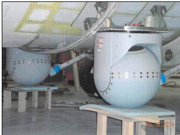
Figure 2 Fix-Mounted MX-20 Cameras on the DEA's ATR 500
