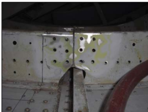
Figure 3 Oblong Holes of the DEA's ATR 500
