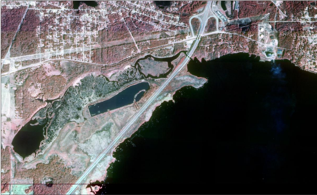
Figure 13. Aerial photograph, 1984, DeBary Bayou and Lake Monroe, stage 2.07 ft. Image following I-4 construction, prior to development of River Oaks Estates, prior to six laning of I-4. Image not to scale in this reproduction.
