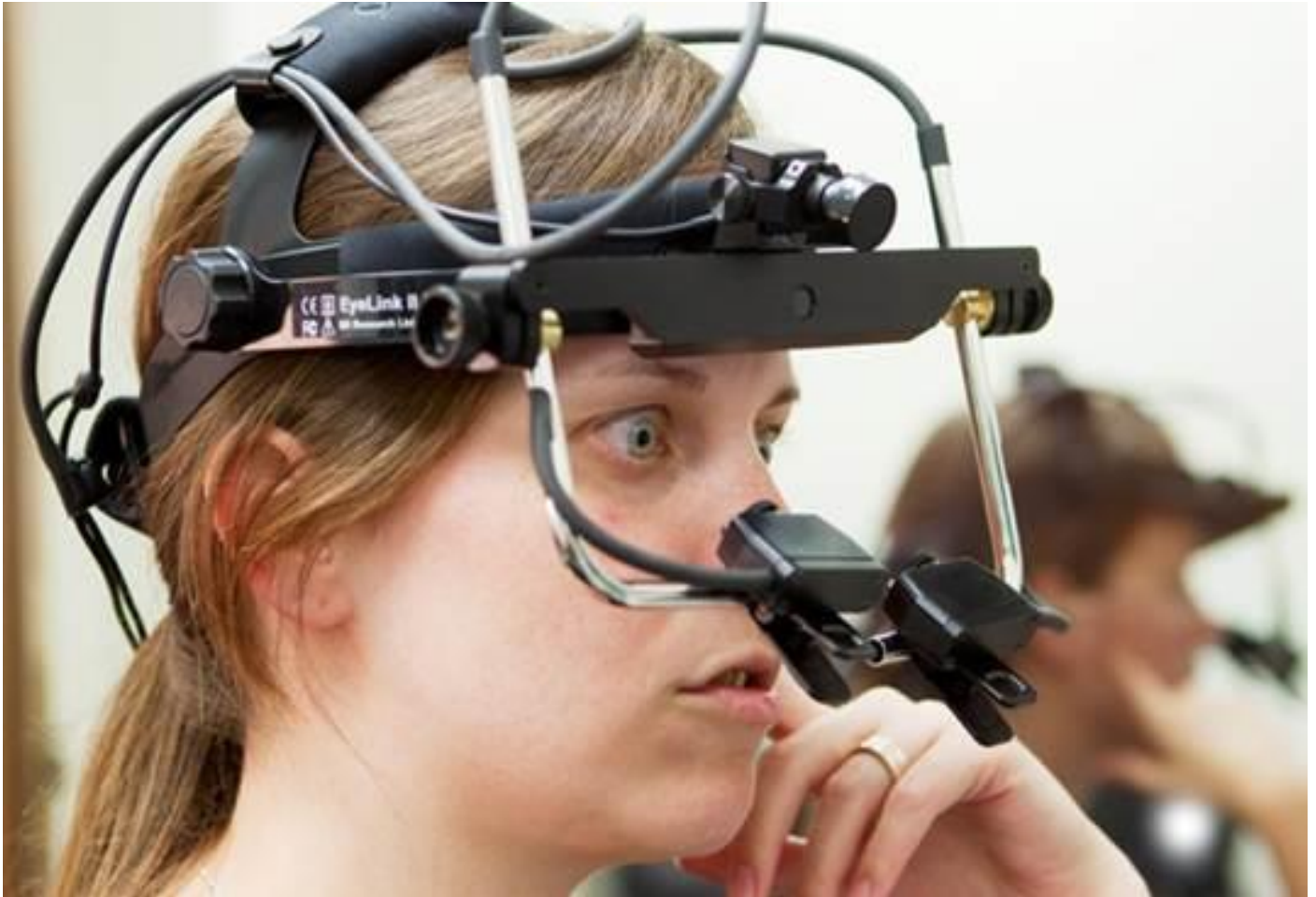
The physical responses of a study participant to disgusting images are measured with an eye tracking device and skin conductance sensors.
