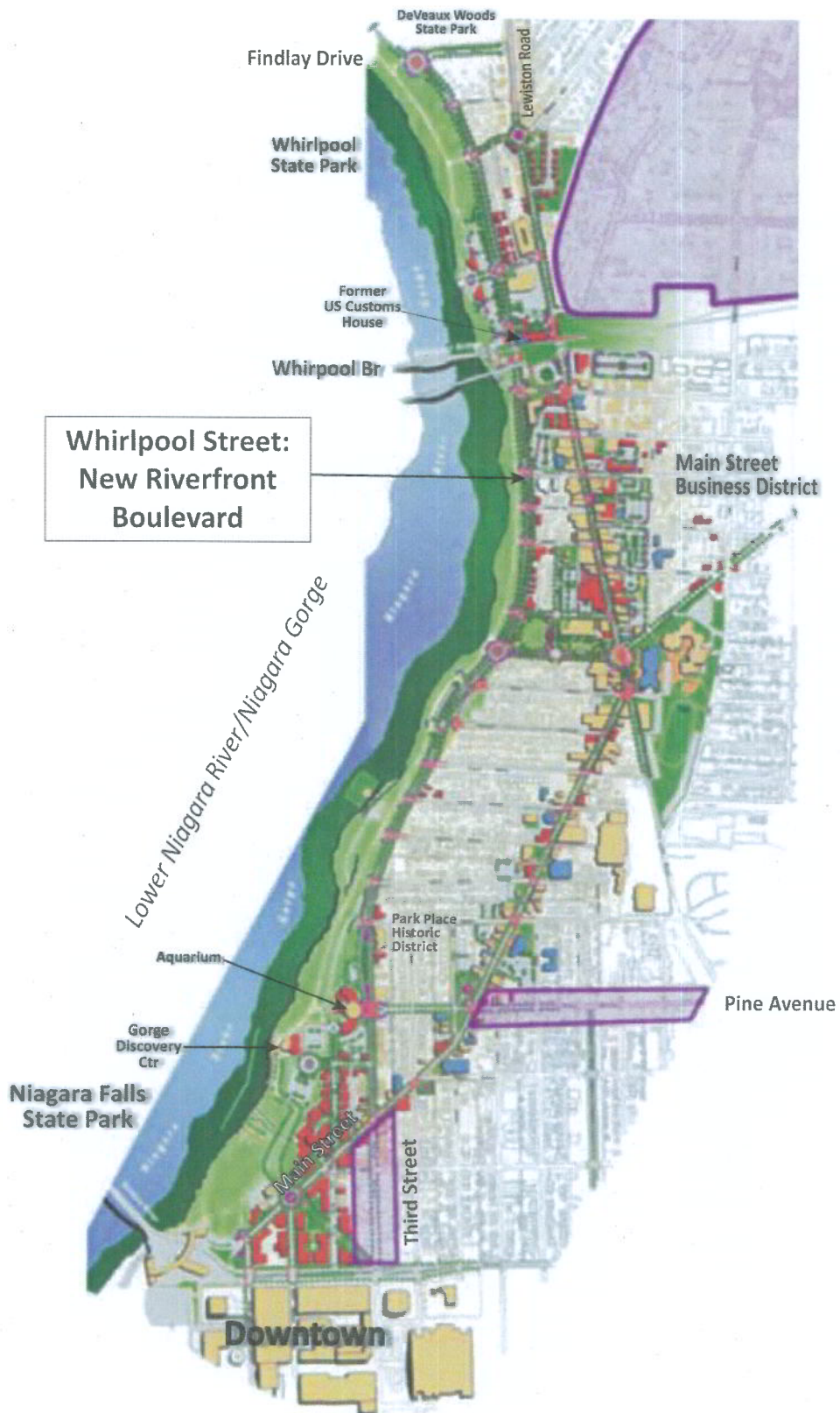
Figure B-3: Concept Design - Reconfiguration of Robert Moses Parkway North/Whirlpool Street, Main Street to Findlay Drive: Originally proposed as part of the Niagara Falls Waterfront Master Plan and later refined in various other plans, the concept would remove expressway features of the RMP North segment and consolidate access along a new Riverfront Boulevard along the current alignment of Whirlpool Street. This would fully open downtown and the City's north end to pedestrian/bicycle access to various park and natural resources along the Niagara Gorge (See also Section in Figure B-4 ).
