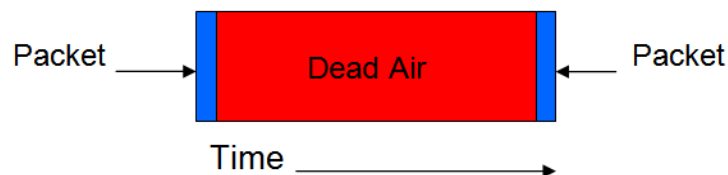
Figure 11 Actual overhead of IEEE 802.11n carrier sensing for single packets sent at high rate. 18
