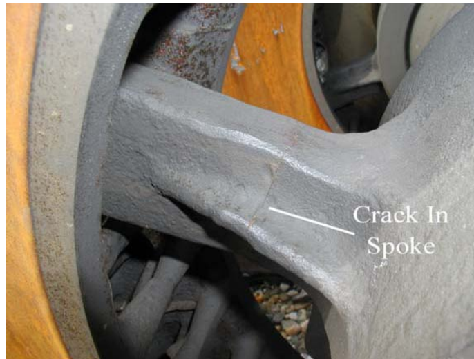
Example of a crack in spoke of WABTEC/SAB-WABCO supplied brake disc used on Acela coach car
