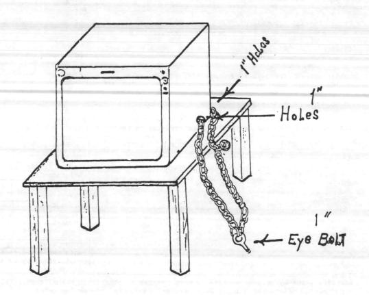
Figure 5-2.--Suggested Method of Securing Television Sets
