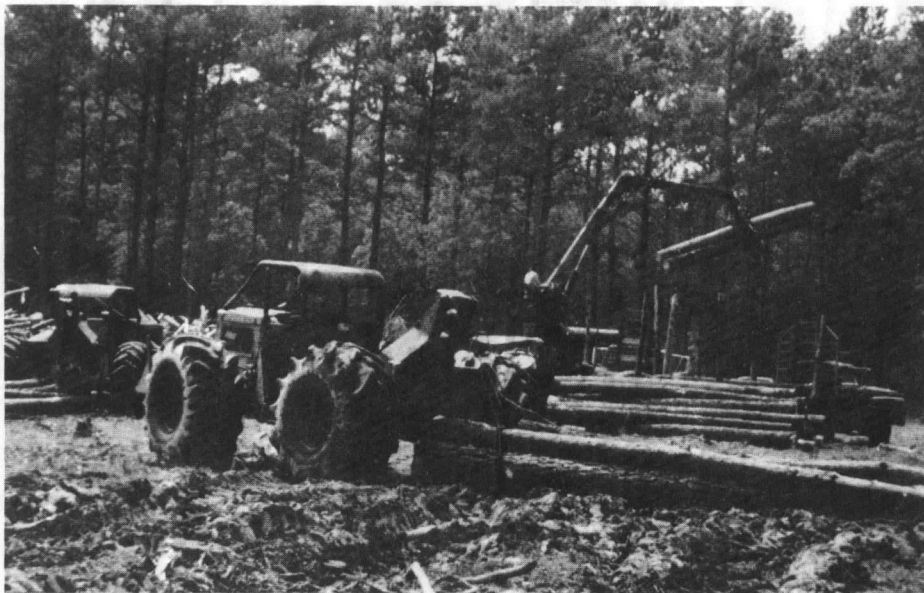
Special wide-tired equipment is required for tree harvest on sites having certain soil restrictions.
