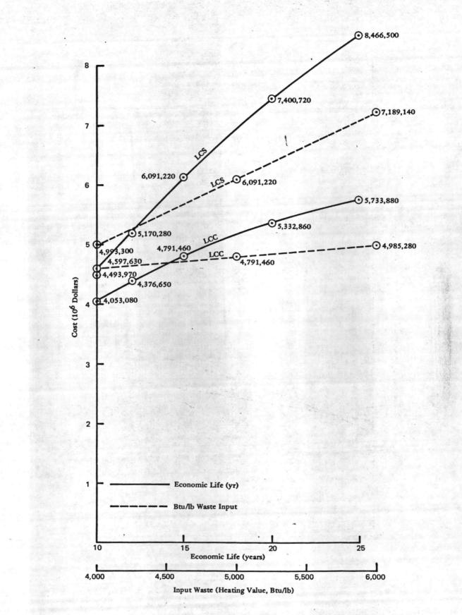
Figure 11. Discounted life cycle cost (LCC) and savings (LCS) versus economic life and input waste heating value.
