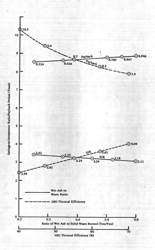
Figure 8. Savings to investment ratio (SIR) and payback period versus ratio of wet ash to solid waste and HRI thermal efficiency.
