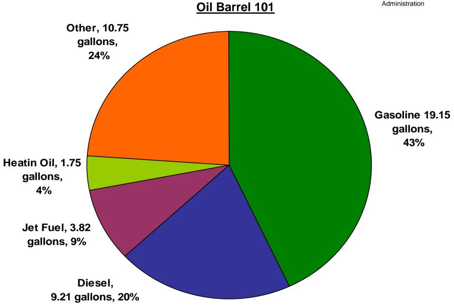
Note: After refining, a 42 gallon barrel of oil nets 44.68 gallons through process gain.
