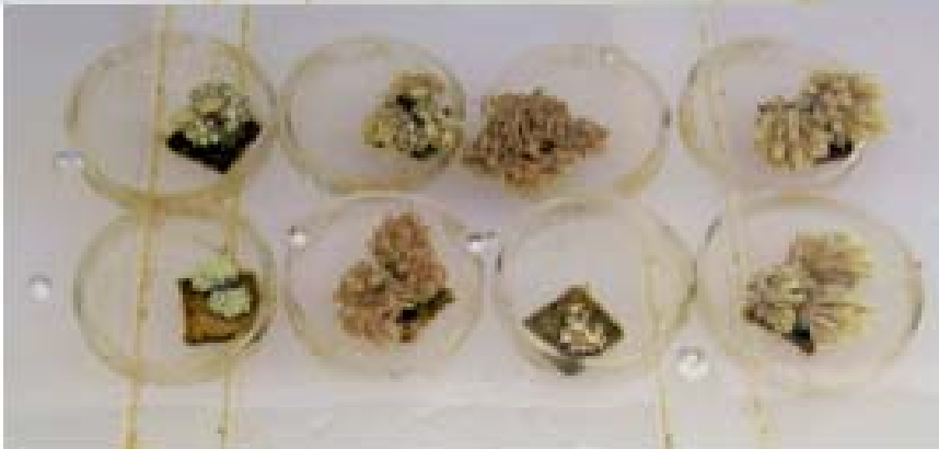
SOFT CORALS EXPOSED TO DISPERSED OIL (using 20ppm Corexit (1:25 ratio dispersant:oil) and 0.5g l -1 weathered Arabian light crude oil with 8 hour exposure).
