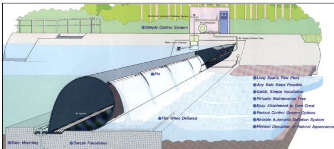
Figure 8 Schematic of Bridgestone Inflatable Dam.
