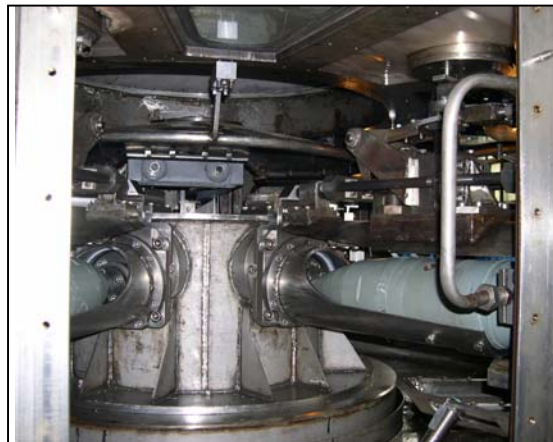
Machine that will drain chemical agent from shells.
