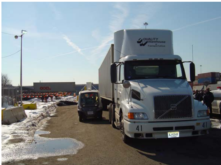
Figure 5. Mobile RPM located at the back of the Smart Cart that is used to determine the source of the radiation. After a truck alarms the RPM located at the entrance/exit to the Port, the truck is sent to the secondary inspection area.
