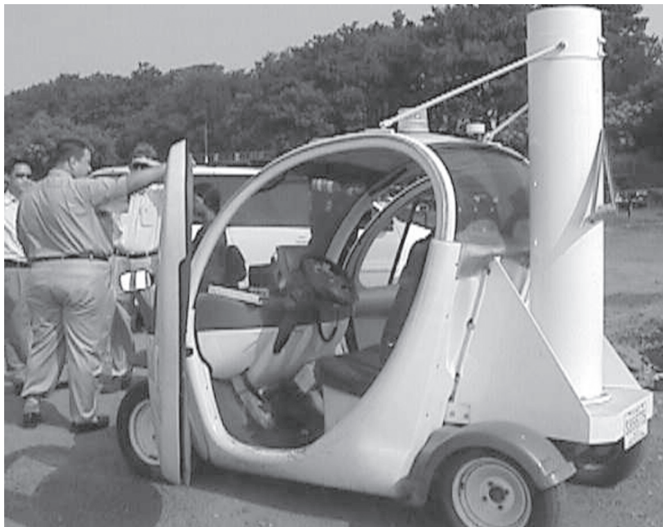
Figure 5: The “SMARTCART,” a Mobile Portal Monitor Using Advanced Detection Technology, Being Tested at the CMTB in New York
