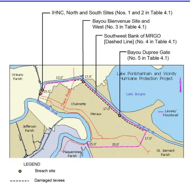
Figure 4.1: Overview map of the Lower Ninth Ward/St. Bernard Parish Polder showing the locations of damage to the primary levee system. Sites nos. 1 through 4 are summarized in Table 4.1. The elevations shown correspond to the top of the levee system at each location (after USACE).
