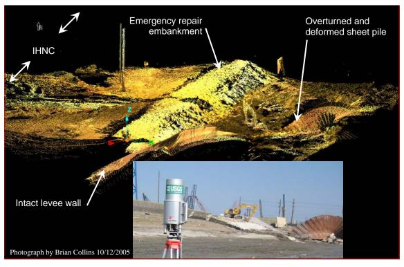
Figure 7.4. For complete coverage of the IHNC-North levee breach the laser was moved around objects that cast shadows. The sheet pile foundation and levee were imaged from both sides to complete the 3-D model.
