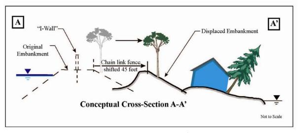
Figure 2.7: Schematic cross section at the 17<sup>th</sup> Street breach section.
