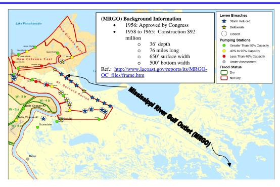
Figure 4.19: Mississippi River Gulf Outlet [MRGO] (USACE). The two yellow stars (i.e., deliberate breaches) along MRGO seem to correspond to locations of gate structures where storm-induced breaches occurred. These yellow stars markers are likely errors in the original map that should have been designated using blue star markers.
