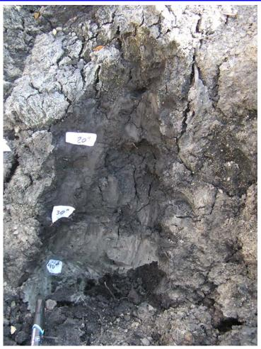
Figure 2.9: Clay seam (light gray layer) underlain by darker lean clay, and overlain by fibrous peat.
