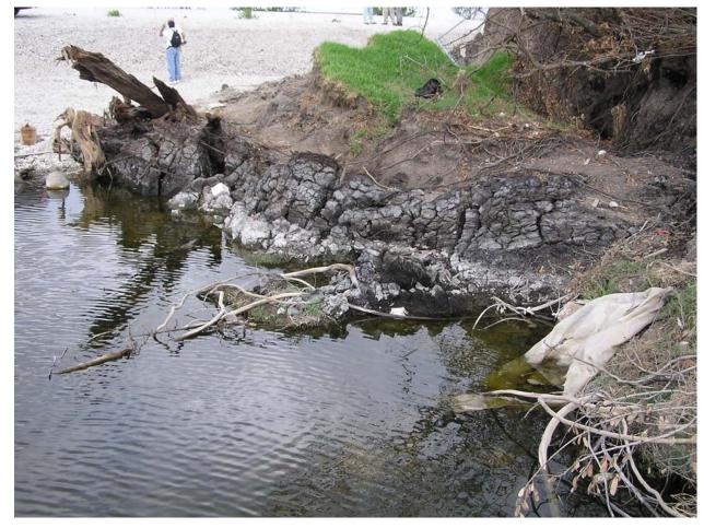
Figure 2.8: Location at which clay seam interbedded within the peat at the toe of the translated levee embankment was sampled.
